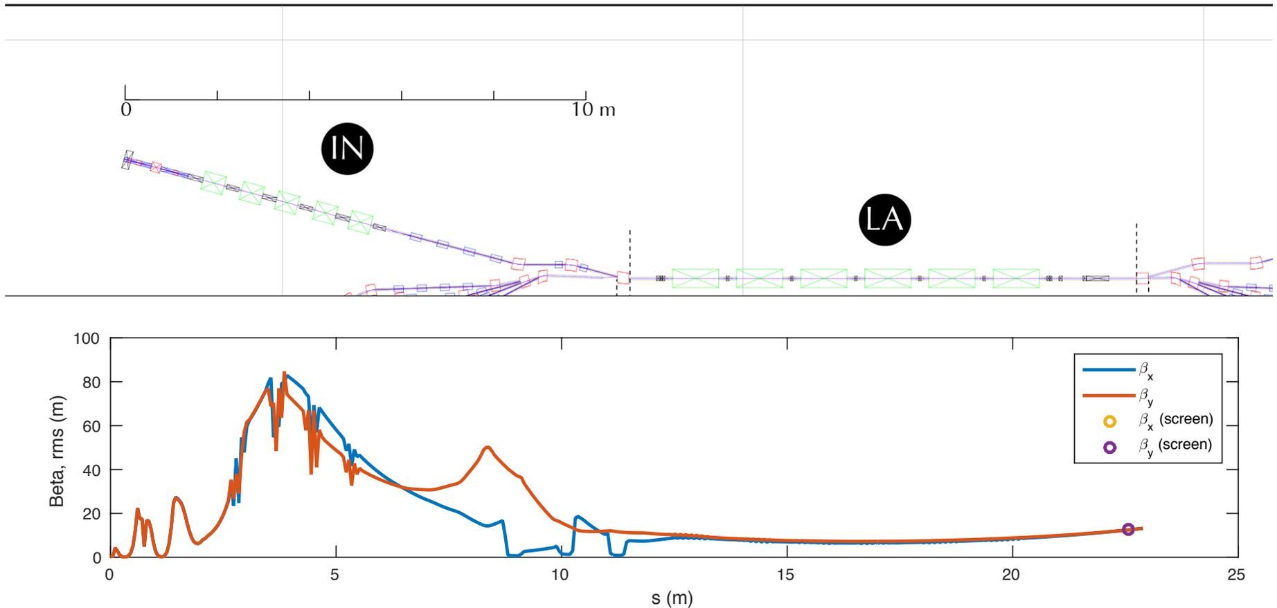
The beam is optimized with space charge using GPT to match specified beam sizes and divergence at the end of the first pass of the Linac.
