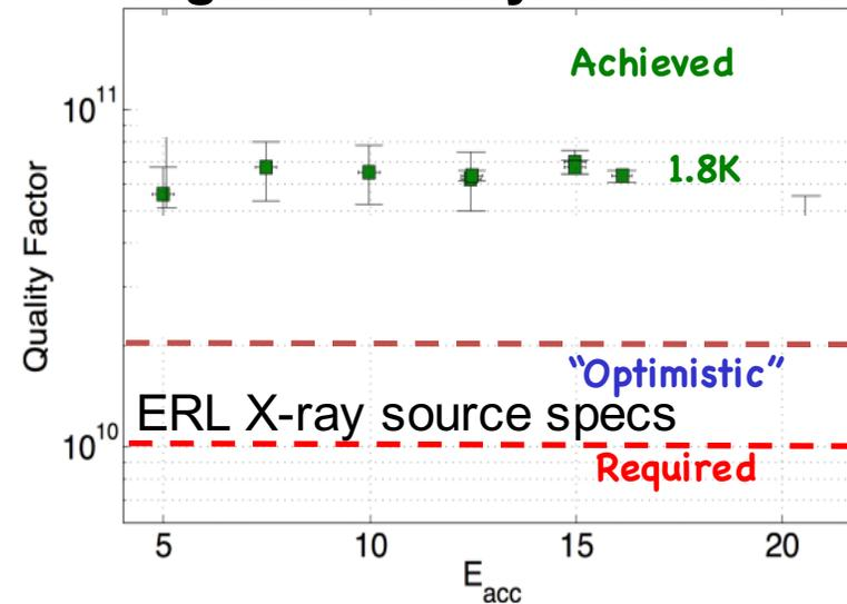
Highest  $Q_0$  in a cryomodule
