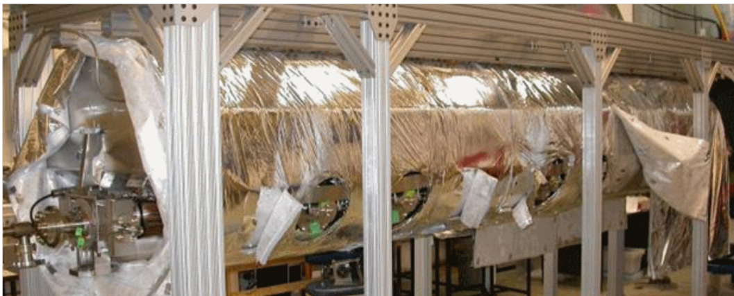
Figure 4.6.14: Photograph of the completed ERL injector 100 K shield being wrapped with MLI.
