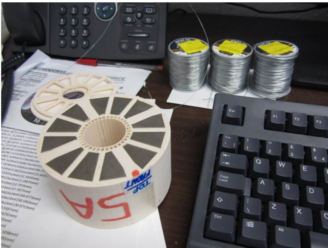
Figure 3.2.16: The pieces of the eRHIC LDRD Halbach magnet placed in a new 3D-printed holder to form magnet “5A”. This is a corrected Halbach quadrupole whose holder incorporates holes for iron shims to be placed around the inside of the bore (iron wire grades shown in background).
