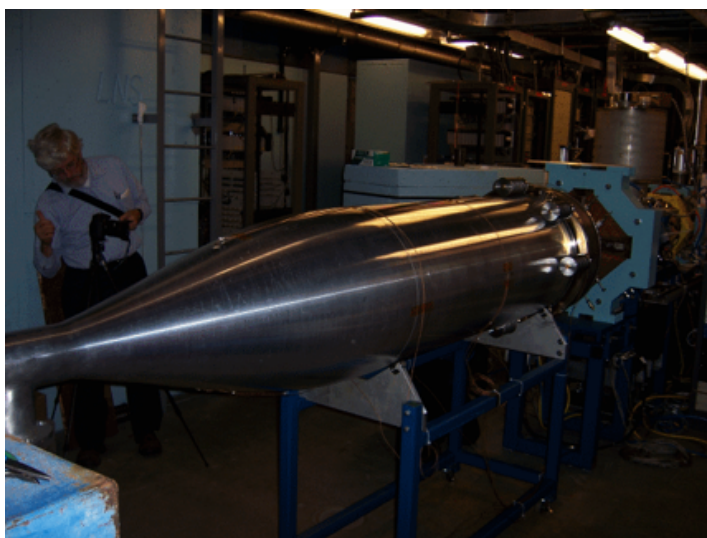
Figure 4.7.2: The completed beam dump before installation of the shielding blocks.
