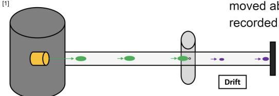
The cropped portion of the beam then passes through to the detector, where its momentum can be ascertained.
