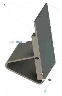
As you can see, there is a joint between the correct two points, but the orientation is funky. To fix this, select "flip" in the Joint window. Use the circular slider to set the correct orientation, then slide the support 0.5" up the face of the support. My assembled joint is shown below.
