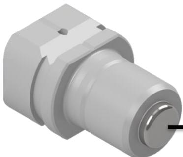
Na-K-Sb grown on molybdenum plug surface
