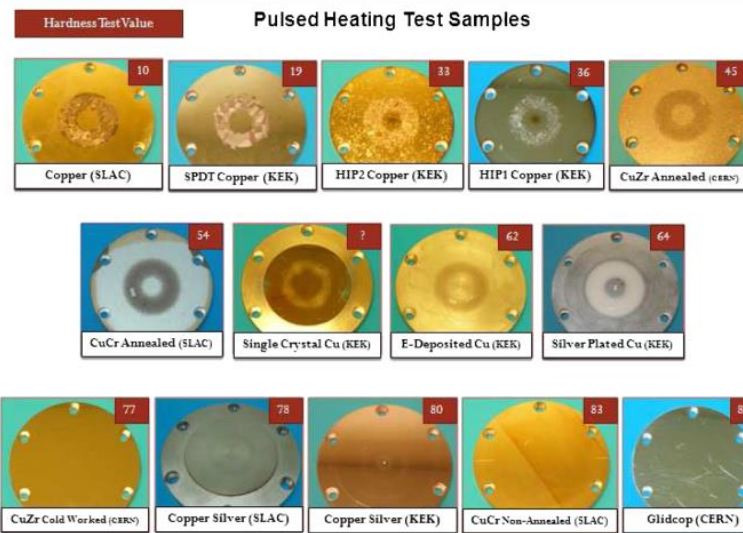
FIG. 54. Pulsed heating samples that have been tested to 110°C. They are listed in order of material hardness values with the softest materials in the top row and the harder materials in the bottom row (hardness values are located in the top right corner of each photograph).
