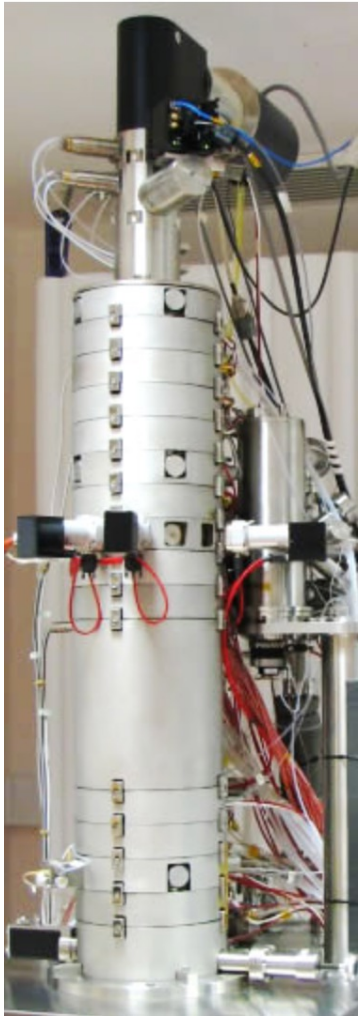
Nion UltraSTEM microscope Atom-scale imaging
