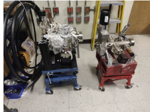
Figure 1. Two suitcases ready for installation/transportation at the UCLA Pegasus laboratory. The one on the right is being shipped back to Cornell to be loaded with cathode. The one on the left has an improved transfer system and it is currently installed on the UCLA Pegasus beamline.
