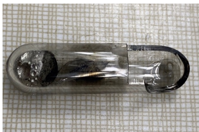
Fig. 1: \sim 5 mm diameter PtSb bead synthesized in a quartz boat prepared by a professional glass blower. The dark deposit to the right of the bead is an Sb film from the cool-down process.
