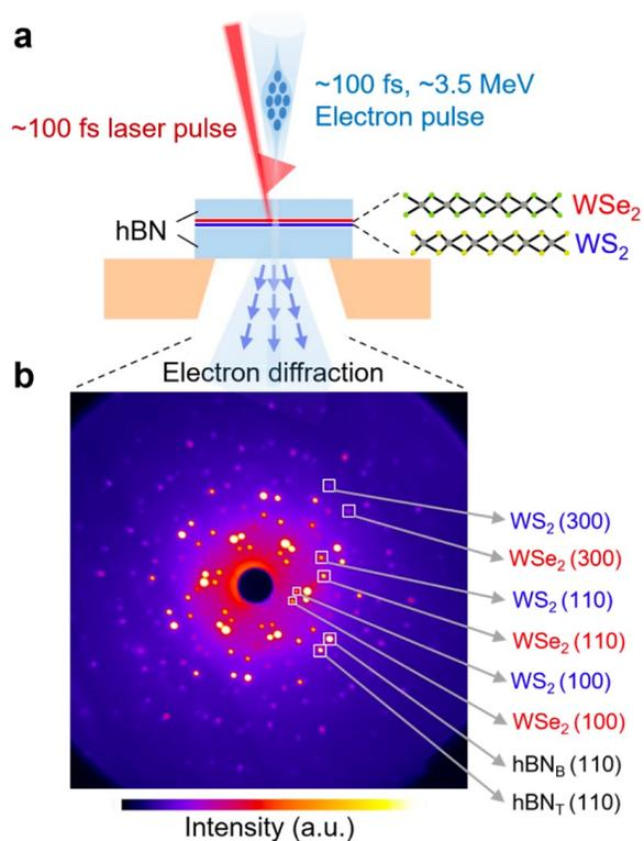
Top: Experimental setup probing dynamic response of 2D van der Waals heterostructures. Bottom: Electron diffraction pattern of heterostructure showing how selective probing of each atomic layer is enabled.
