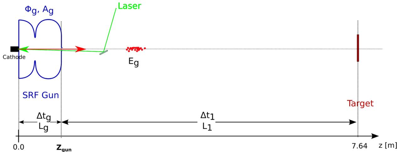
The electron bunches sample different fields than the nominal in the gun. The reasons are:
