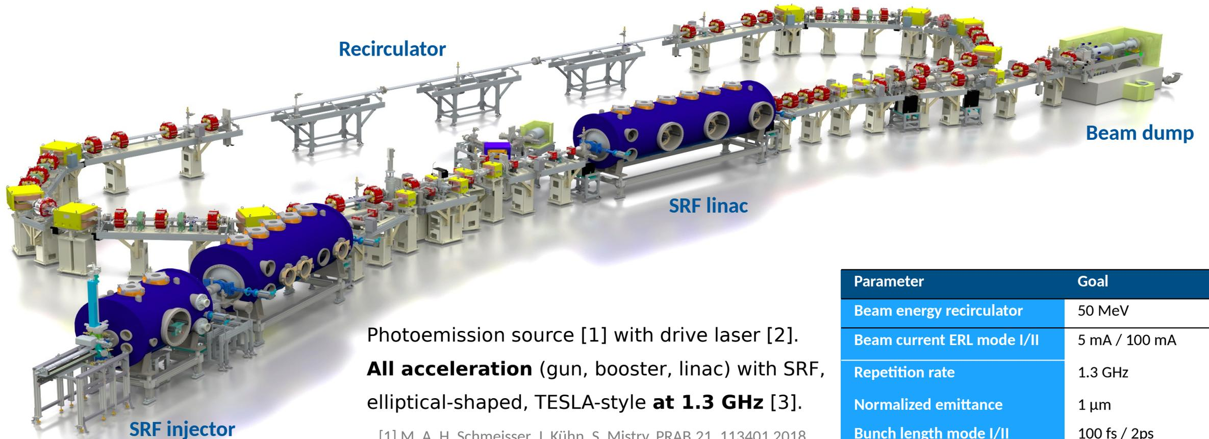
Photoemission source [1] with drive laser [2].
