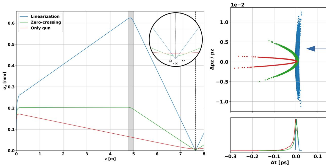
Linearization using the stretcher mode [1] provides the shortest bunch at target.
