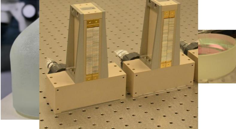
Diode-Pumped Tm:YLF Multi-Pass Amplifier
