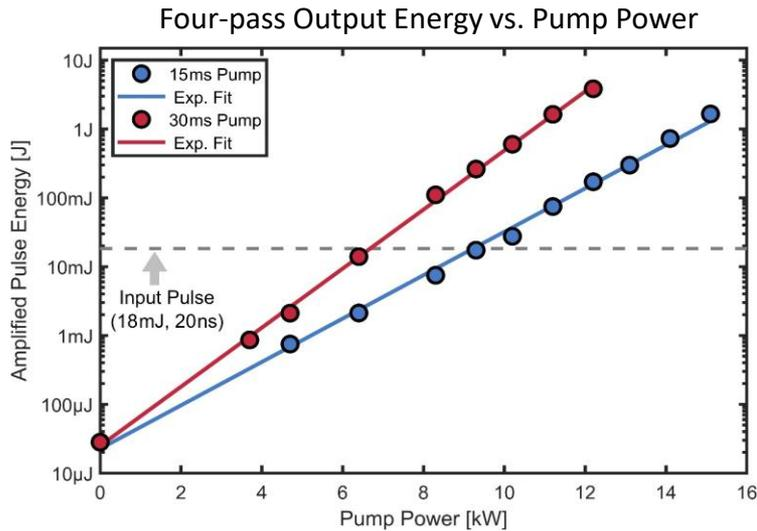
Diode-Pumped Tm:YLF Multi-Pass Amplifier
