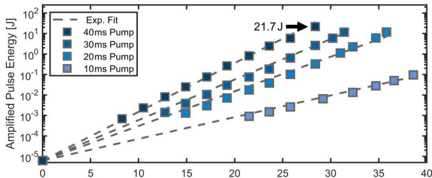
6-pass amplified pulse energy (long pulse)
