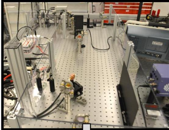
Diode-Pumped Tm:YLF Multi-Pass Amplifier
