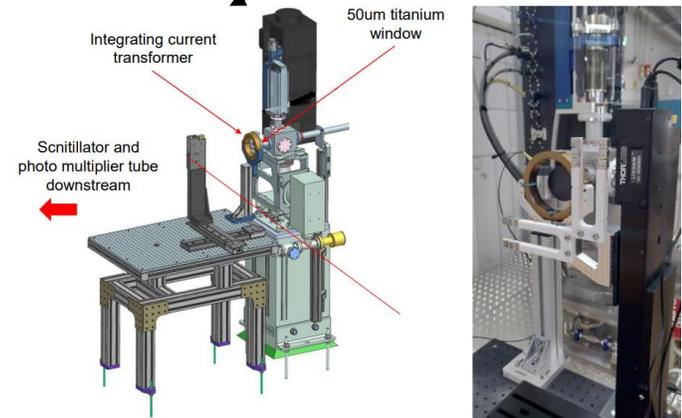
*Equipped with exit window, wire scanners (both planes), screen and ICT. Upgrade with quadrupole triplet and steerers planned.*
