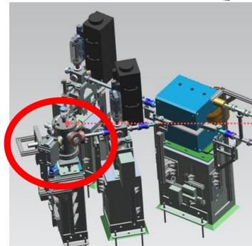
*In the dispersive section Equipped with mover. No UHV requirements.*
