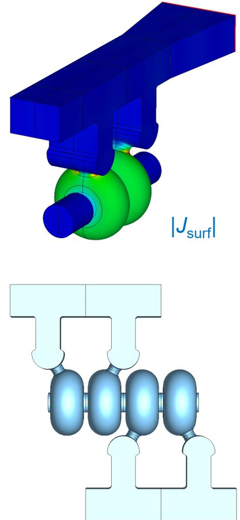
CST calculated fields and power in the test cavity
