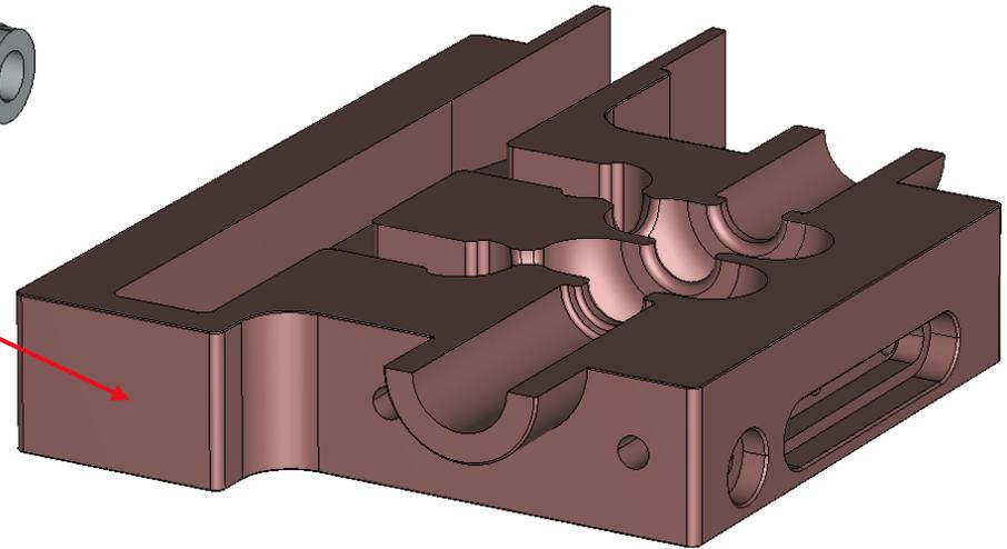
C-band test cavity: CAD model and machined half-structure (picture top right)
