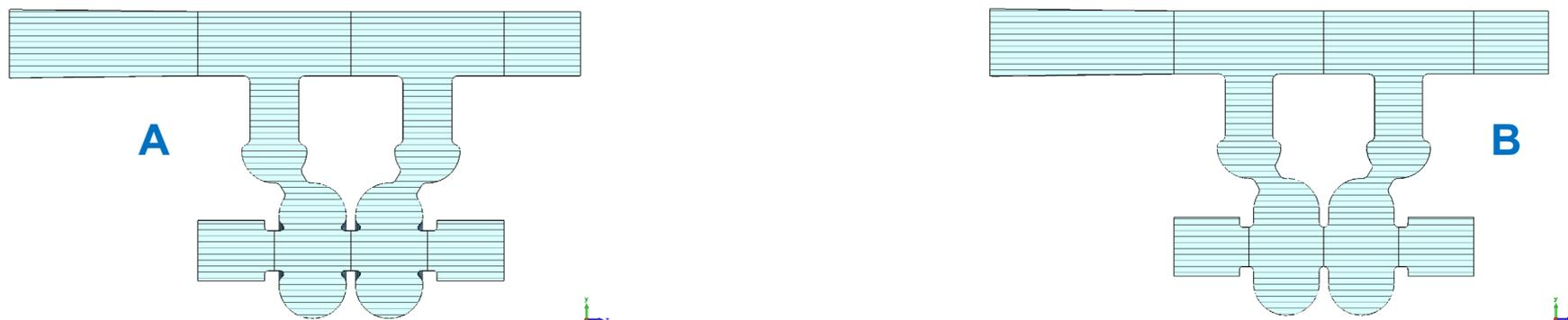
Comparison of two cavity types.  $f = 5.712$  GHz; ideal Cu;  $E_0 T = 80$  MV/m
