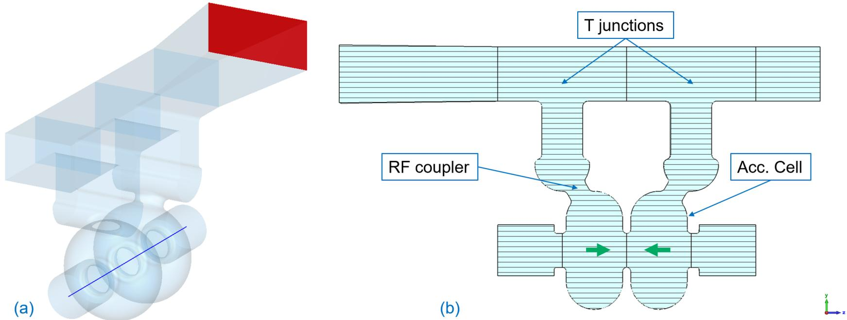
C-band 2-cell  $\pi$ -mode test cavity for  $\beta = 0.93$  (1.6-GeV protons): (a) inner vacuum volume with standard WG187 port (red); (b) vertical cross section.
