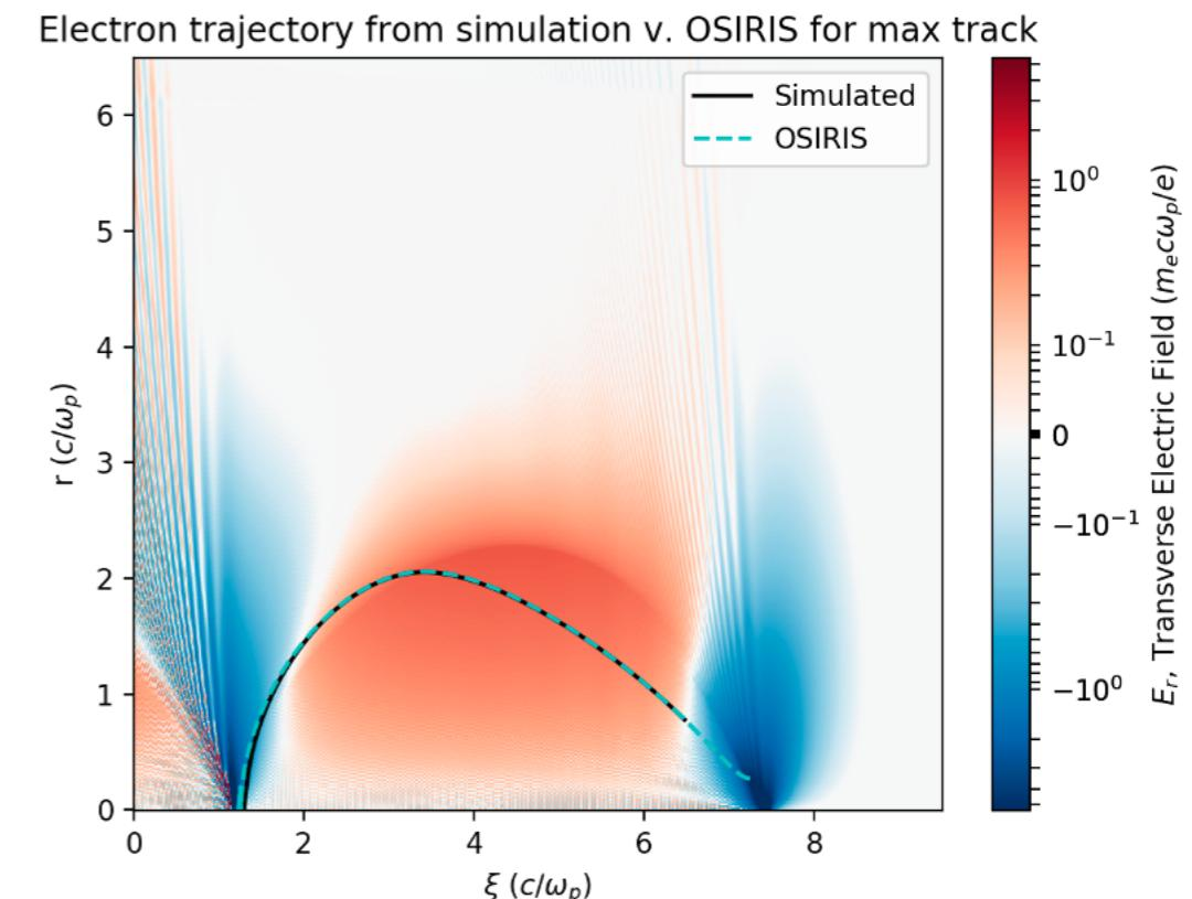
The performance was checked by comparing eTracks trajectory with OSIRIS trajectory\*
