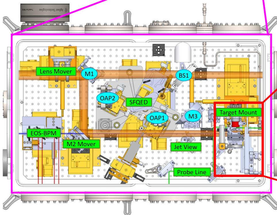
Target mount with 1 urad tip/tilt resolution.
