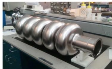
Potentially dangerous HOMs were identified and classified until 2.4 GHz. A trapped monopole mode was found at around 2.25 GHz
