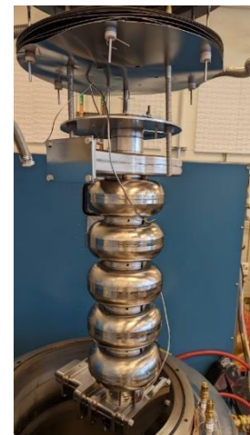
C75 cavity made from large grain Nb
