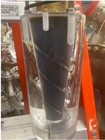
Custom designed HV plug with cooling channel
