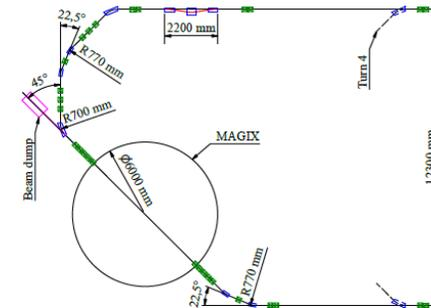
Figure 1.4: Sketch of the beam line for the internal experiment MAGIX.
