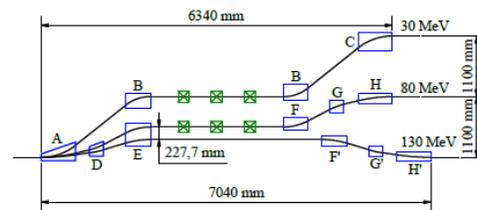
Figure 1.2: Sketch of the beam separation for uneven turns.
