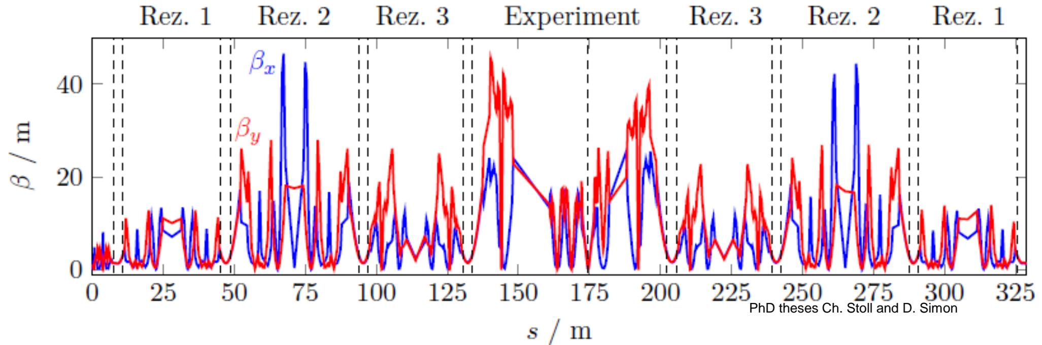
ERL-Lattice – not completely symmetrical due to energy (gain) dependent focussing of RF-structures.
