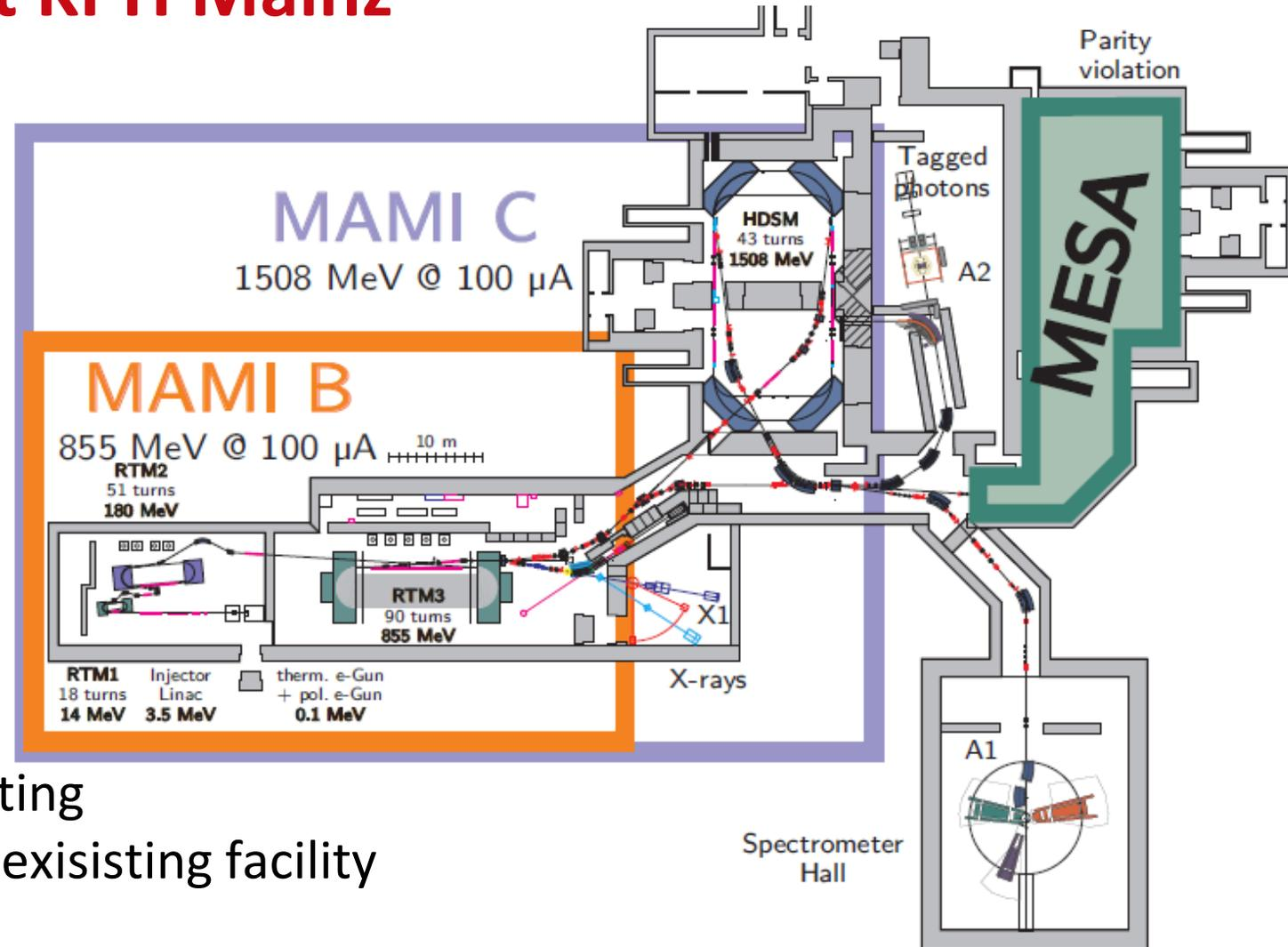
Mainz Energy Recovery Superconducting Accelerator (MESA) to be built in the existing facility
