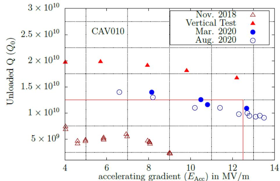
Cryomodules miss dynamical specs slightly but fulfill static specs by wide margin
