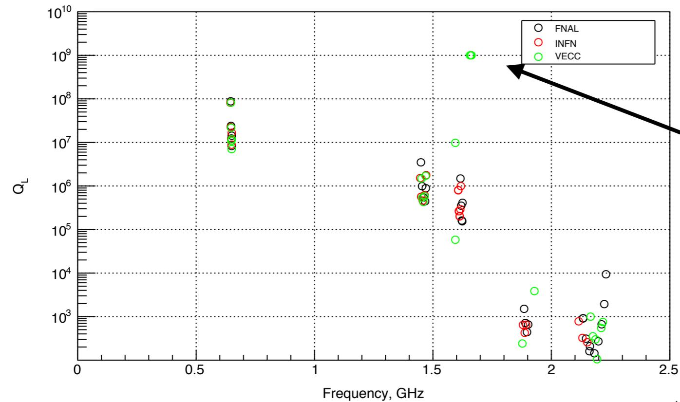
Dangerous trapped mode in VECC design:  $f=1.663$  GHz,  $(R/Q)=18$  Ohm
