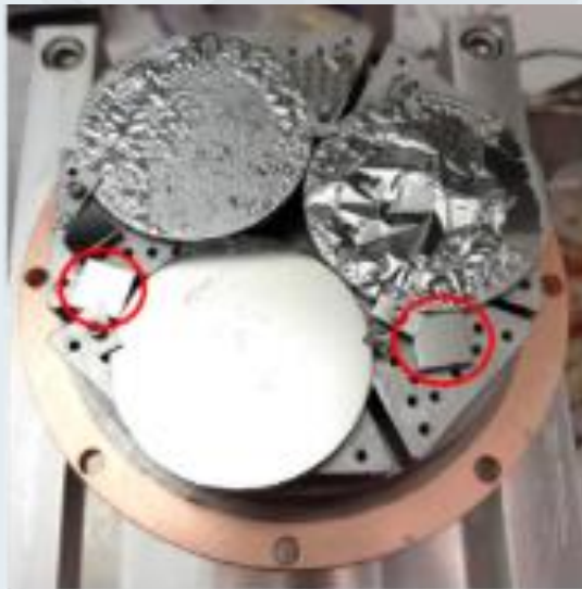
Samples in chamber after Nb film deposition @ -120V
