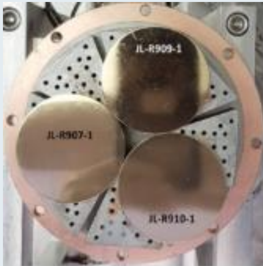
Samples in chamber prior to Nb film deposition
