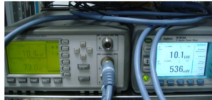
Maximum tested power: 10 kW, CW
