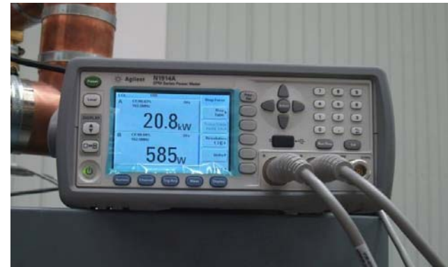
Maximum tested power: 20 kW, CW
