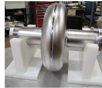
3 JLAB \beta=0.6 cavities, 100mm iris with, 0 degree
