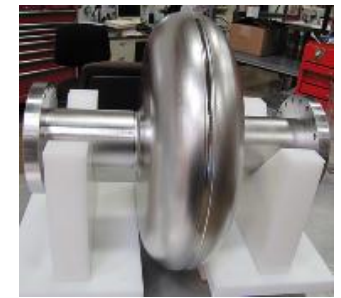
3 FN AL \beta=0.6 cavities, 86mm iris with, 1.9 degree
