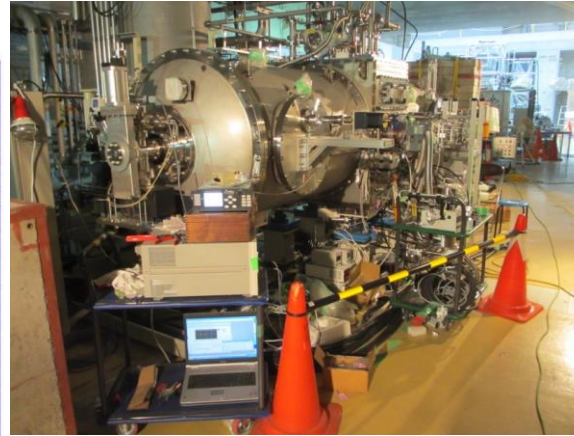
ERL Main Linac Cryomodule High Power Test (Radiation on axis vs Vc)
