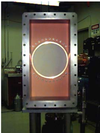
PEP-II 476 MHz waveguide window assembly
